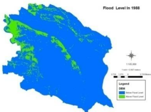
Figure 2 (d): Flood map of 1988 Prepared from Three Dimensional (3-D) Satellite Image
